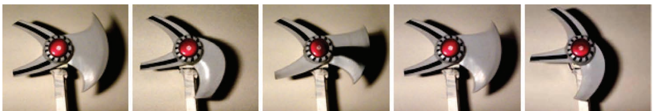
Figure 2. Examples of deformation of symmetrical images three-blade propeller rotating at a speed of 6-8 rps (shooting was done with a short shutter speed of 1/2000 s)
