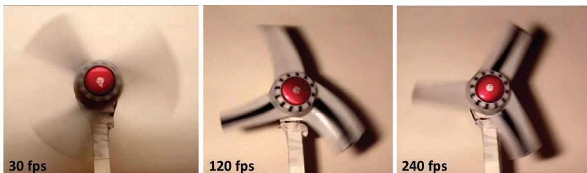
Figure 1. Images (still frames) of rotating blades of a symmetrical fan at different shooting frequencies and standard (automatic) mode settings
